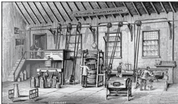
15. In this stylized engraving of a nineteenth-century dairy factory, every machine is connected by a belt to the same driveshaft.
